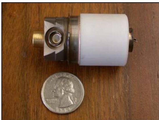
Figure 8; Oxford Instruments X-ray Technology Inc. miniature field emission X-ray tube with gated MWNT 2mm diam. cathode.
