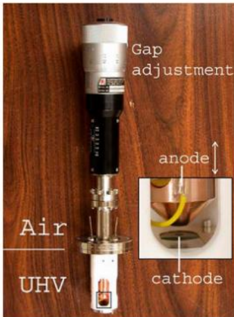
Figure 5; instrumental setup for field emission characterization.
