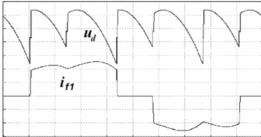
Figure 19. Voltage on the load and phase current influenced by firing pulses non-symmetry
